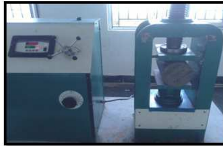
Figure 4.3: Split Tensile Test for Concrete Cylinder
