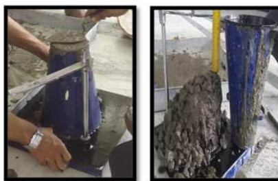
Figure 3.1: Slump Test for Fresh Concrete
