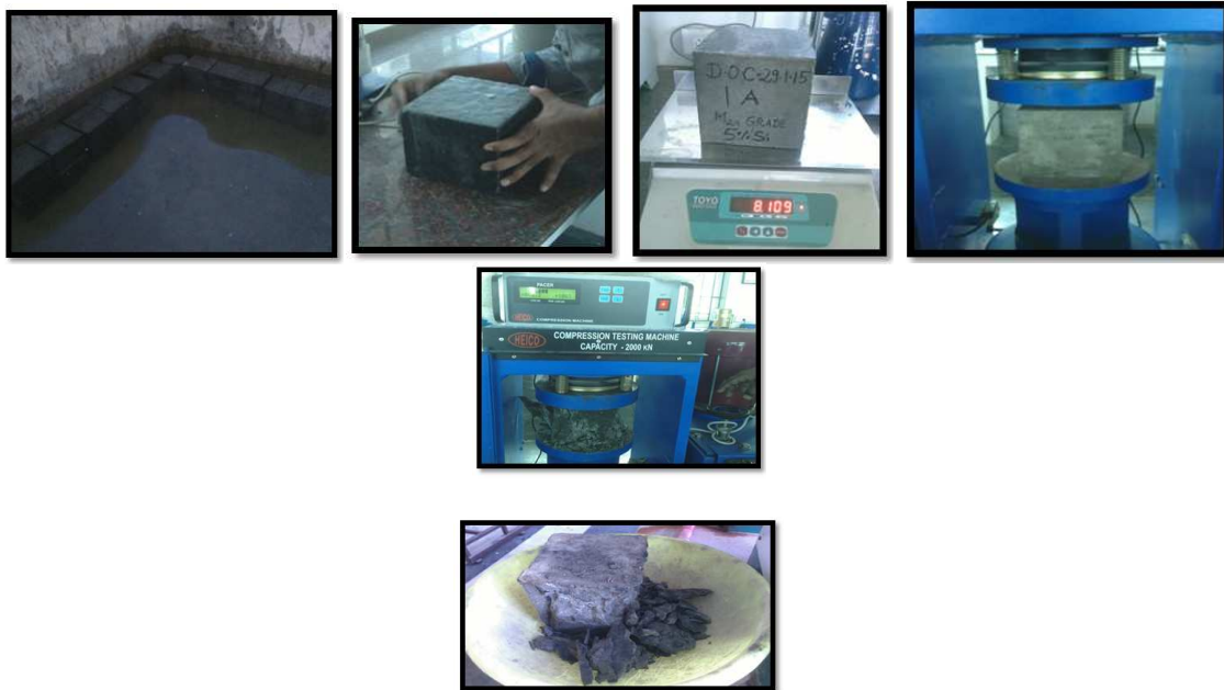
Figure 4.2: Cube Curing and Testing
